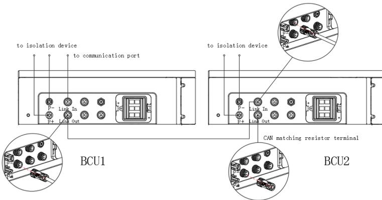
Notes: BCU1 is the first group of batteries;BCU2 is the second group of batteries, and so on, coded sequentially.
